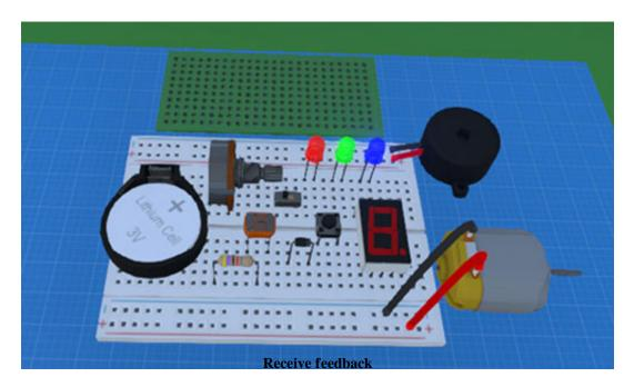
Get information about circuit components values (voltage, current, voltage drop, resistance, ...) when hovering over them with the controller. Easily detect errors in your circuit as you'll get a warning when doing something wrong (short circuit, open circuit, too much current, ...).
